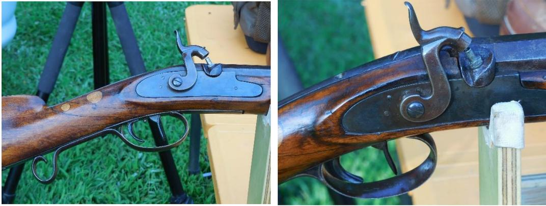
Note the repaired wrist and the rounded lock plate inlet. The tail ends on some rifles were pointed at the rear. This is a replacement lock and hammer. The originals were lost. The breach plug has a long tang but is not a hook breach.
